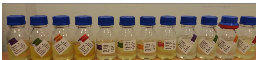
Figure 11 Liquid product samples for 12 reaction conditions. Lighter colour is observed at higher severity, which corresponds to greater HDS and HDA
