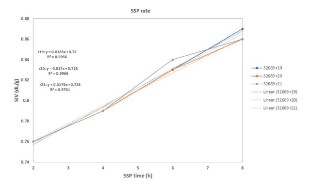
The SSP rates for both TEST variables are within the EPBP specification with a deviation below 10% vs CONTROL.
