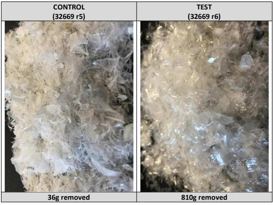
Only PET fines have been removed for the CONTROL variable. When it comes to TEST variable, what has been collected are thin flakes where it is not possible at this step to identify the structure (1, 2 or 3 layers) and composition (PET, PEF or PET/PEF).
