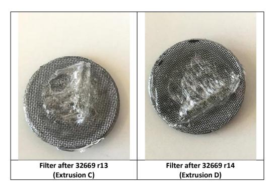
The extrusion process went very well with no flakes sticking, feeding issues, fumes or strange odors. No residues have been found on the filters after the processing of each variable described above.
