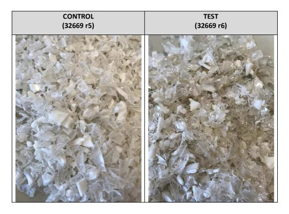
A slight discoloration (yellowing) has been observed on the TEST variable. The Oven test results demonstrates that the PEF layer has not been completely separated from PET by the grinding, washing and air elutriation steps.
