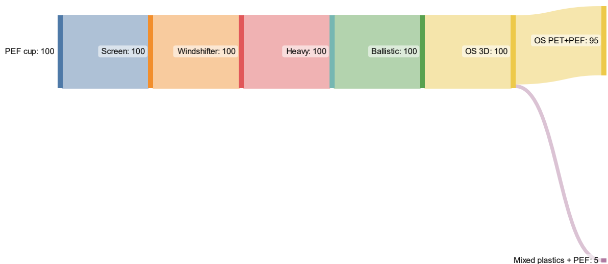
Figure 16 Sorting behaviour of PEF-3 when PEF is sorted together with a PET stream
