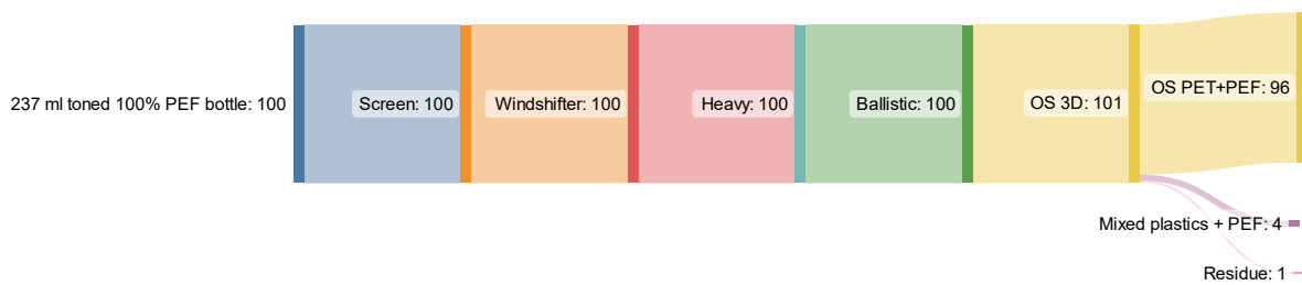
Figure 19 Sorting behaviour of PEF-4 when PEF is sorted together with a PET stream
