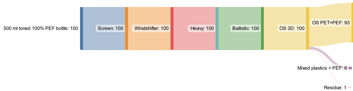
Figure 22 Sorting behaviour of PEF-5 when PEF is sorted together with a PET stream
