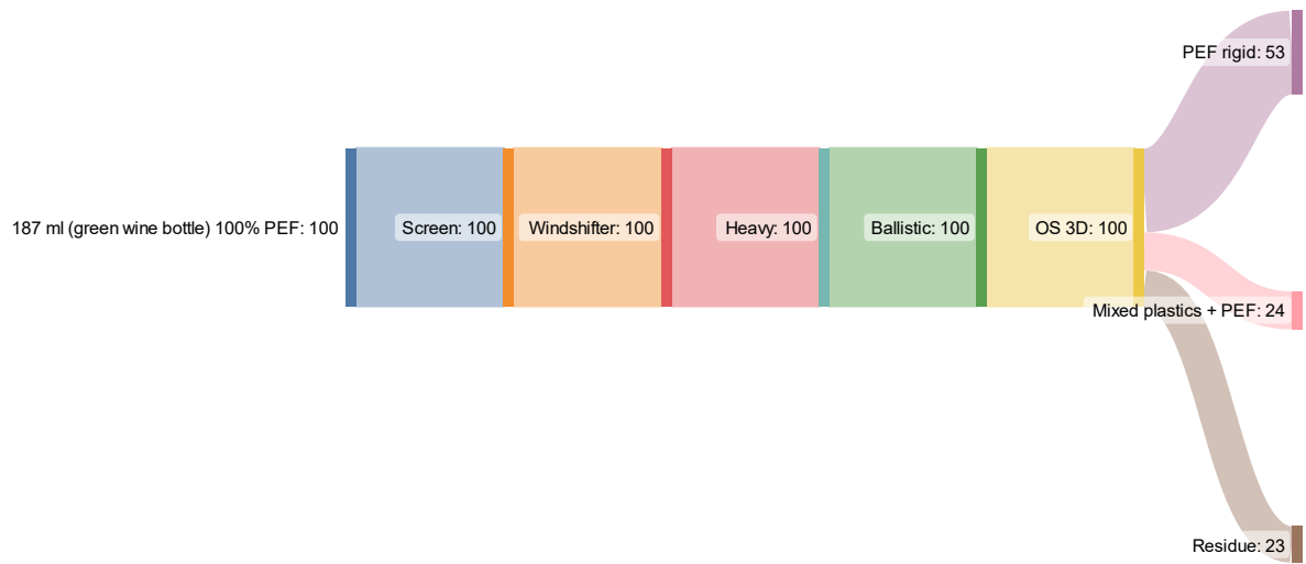
Figure 29 Sorting behaviour of PEF-7 when PEF is sorted as a separate stream
