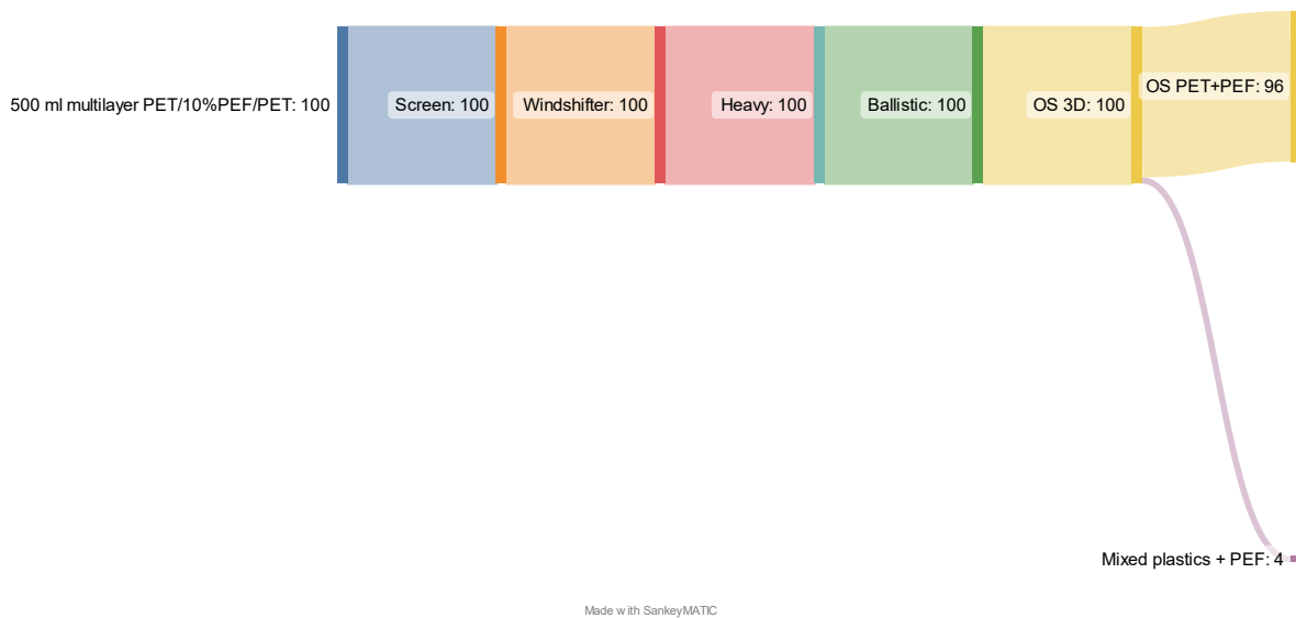
Figure 11 Sorting behaviour of PEF-1 when PEF sorting together with the PET stream
