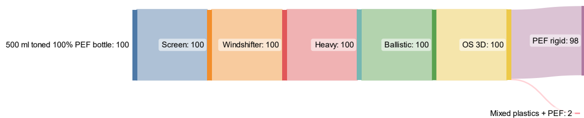
Figure 23 Sorting behaviour of PEF-5 when PEF is sorted as a separate stream
