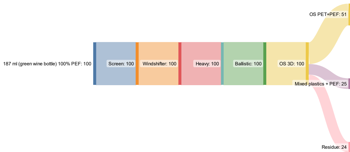
Figure 28 Sorting behaviour of PEF-7 when PEF is sorted together with a PET stream
