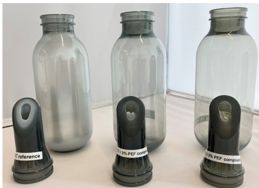
Figure 5. The preforms and bottles produced from full rPET, rPET + 2 wt% PEF and 5 wt% PEF (from left to right). The preforms were cut open at a 45° angle from the longitudinal axis, and the surface was polished to visualize the haze/crystallization through the thickness of the preform wall.
