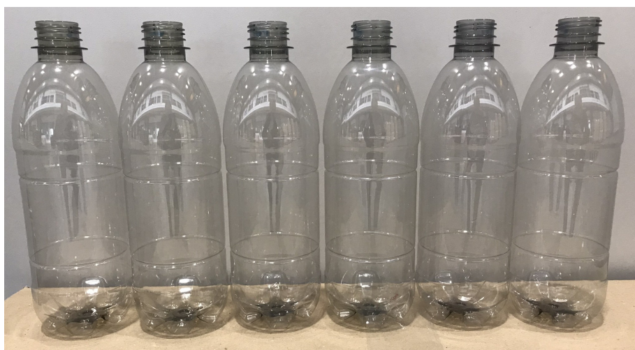
Figure 4. Visual appearance of the 500 mL bottles produced from the rPET resins produced in a commercial recycling process. From left to right, the bottles are produced from rPET with 10 wt% PEF, 5 wt% PEF, 2 wt% PEF, 0 wt% PEF (reference), 5 wt% PEF + toner and 10 wt% PEF + toner.
